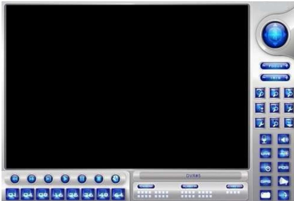
The video images can be displayed in several types of split-window screens, including 1/4/9/16-Window for single DVR and 25/36/49/64 for multiple DVRs. And the focus window is surrounded by a frame border. In addition to the video windows, there are different icons on the lower corner and the right corner of the screen for status display and control.
